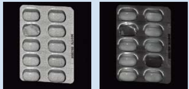
The intensity image of a blister pack to the left and the scatter image to the right. Note how two cells of the blister pack are much darker in the scatter image. This indicates that pills are missing in these cells, something which is not possible to conclude from the intensity image.
