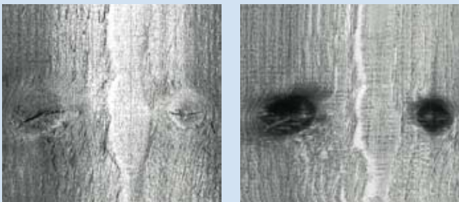
The intensity image of a board to the left and the scatter image (Tracheid) to the right. Note how the knots in the scatter image appear much darker than in the intensity image, thus making the knot identification much easier and more robust.
