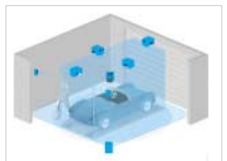
Fig. 1-9: Checking overhang in automated multi-storey car parks
