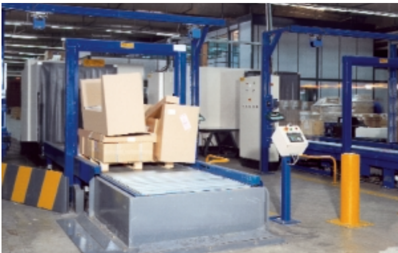
VMS 200: Determining the volume of air freight with irregular contours.
