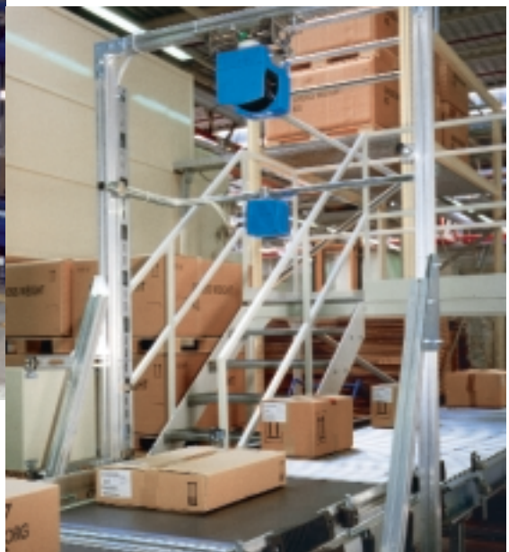
VMS 100: Determining volumes for automatic storage.
